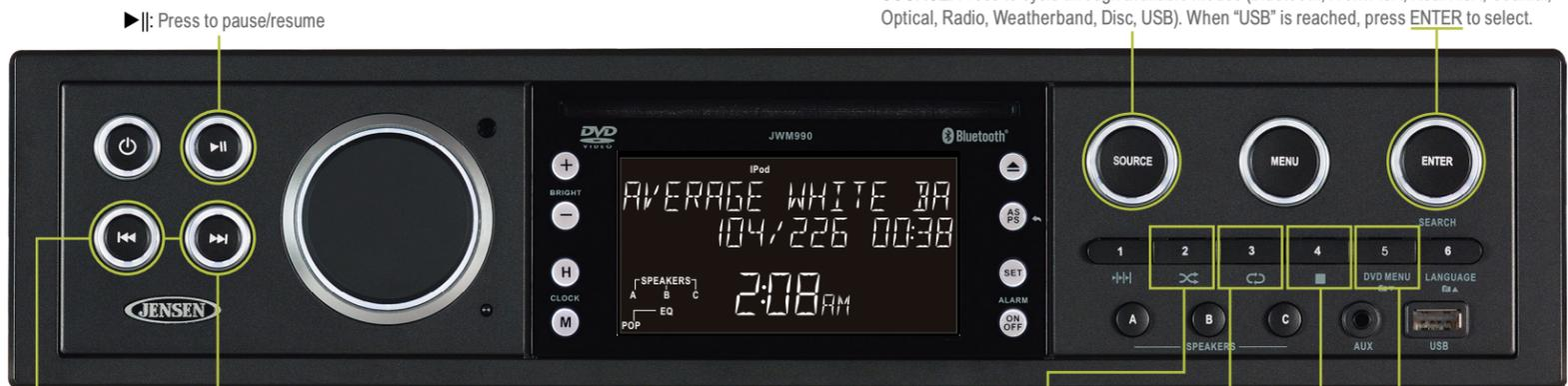
**PREV TRACK:** Press once to go back to the beginning of current track, twice to play the previous track, or press and hold to fast reverse seek through the track.
