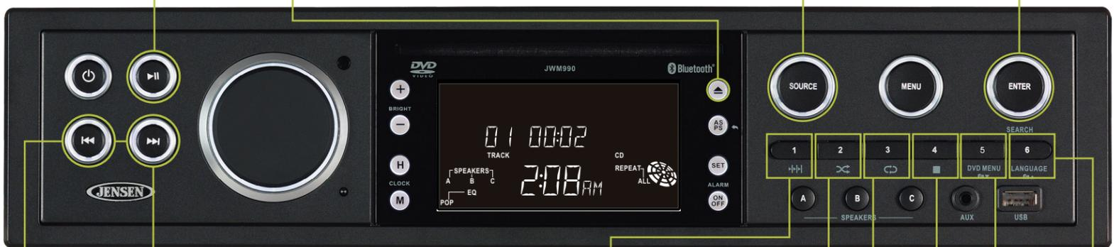
**PREV TRACK:** Press once to go back to the beginning of current track, twice to play the previous track, or press and hold to fast reverse seek through the track.
